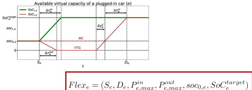
MC ... Managed Charging VTG ... Vehicle-to-Grid
