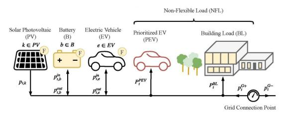
This case study examines the potential value that the flexibilization of the technologies of an Energy Management System may create in a period of one year.
