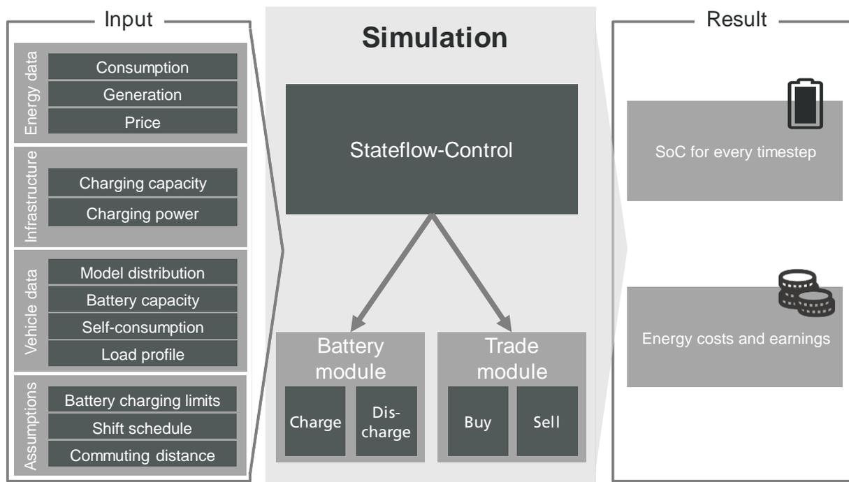
Figure 1: Structure of the simulation model (middle) with its inputs (left) and target figures (right)
