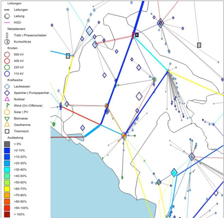
Figure 1: Capacity utilisation of the transmission network in Montenegro, 2040 (Scenario 2)
